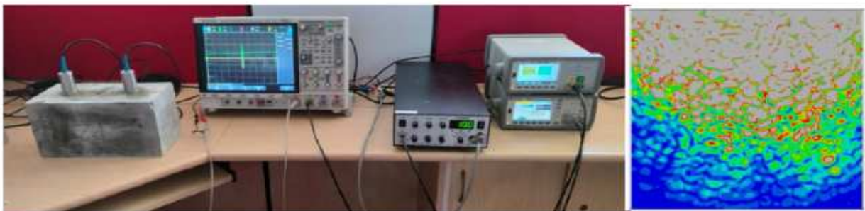
Fig. 3. Ultrasonic set-up to perform micro structural study in cementitious specimen and the wave-matter interaction using numerical model
