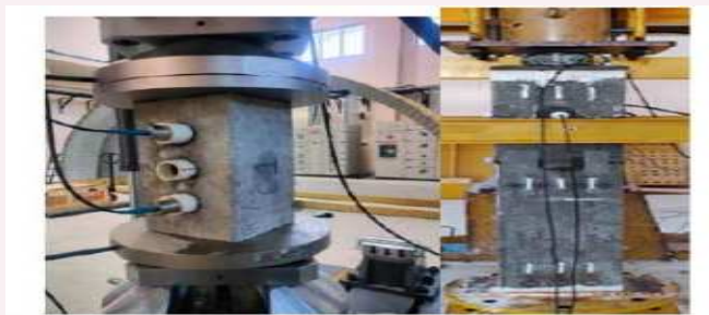
Fig.6. Experimental set-up for stress state monitoring in prism specimen and axial concrete member.
